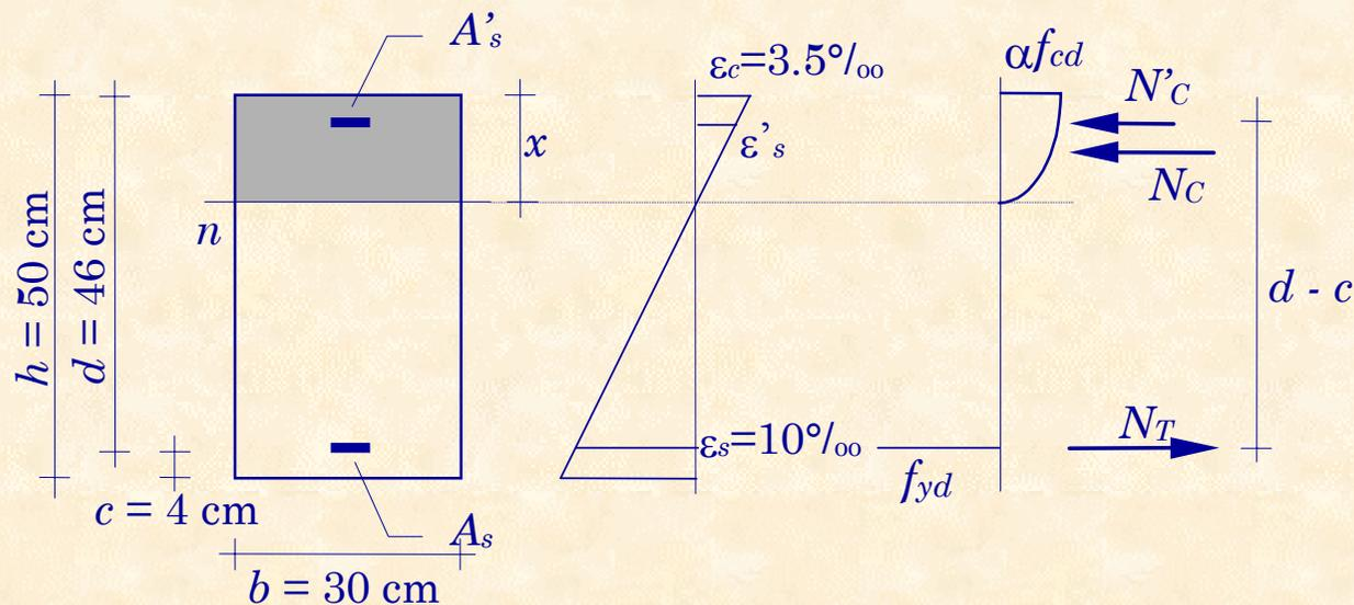
$$M_o = \frac{d^2}{r_{slu}^2} b = \frac{0.46^2}{0.0220^2} \times 0.30 = 131.2 \text{ kNm}$$
