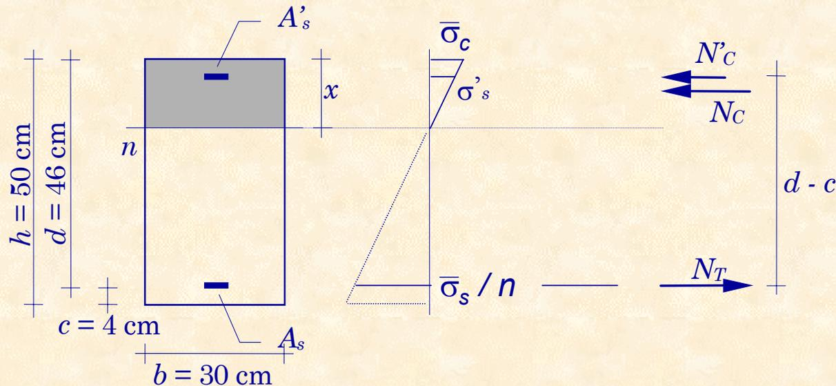
$$M_o = \frac{d^2}{r_{TA}^2} b = \frac{0.46^2}{0.0282^2} \times 0.30 = 79.8 \text{ kNm}$$
