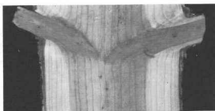
The lateral branch is connected to the pith of the main stem. Each successive growth ring or layer forms continuously over the stem and branches.
