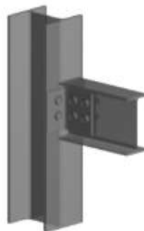
Hybrid (welded flange/bolted web) site connection
