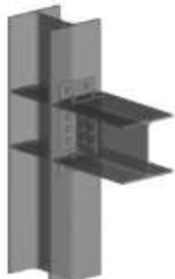
T-sections with preloaded bolts to flanges
