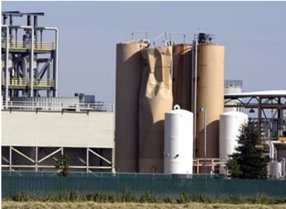
Silo collapse due to vacuum
