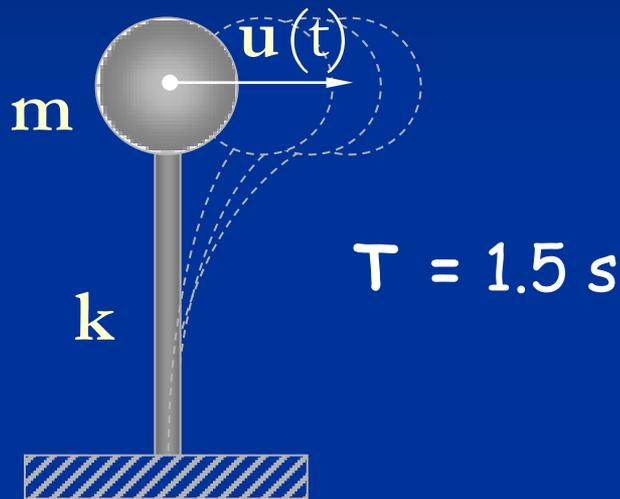
$$m = 73.320 \quad \text{kN s}^2/\text{m}$$
