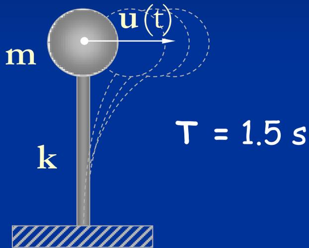
$$m = 73.320 \quad \text{kN s}^2/\text{m}$$
