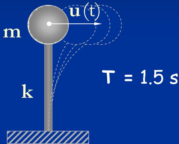
$$m = 73.320 \quad \text{kN s}^2/\text{m}$$
